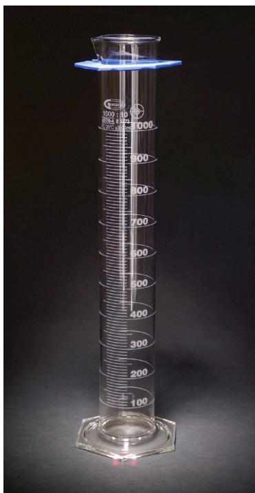
Graduated cylinders are very useful when measuring precise volumes of liquids.
