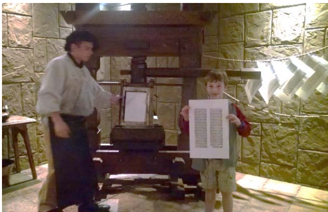
This is a replica of Guttenburg's press. The boy is holding a sample page made on the press.
